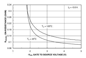
Figure 3. On-Resistance Variation withTemperature.
