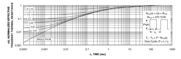
Figure 11. Transient Thermal Response Curve.
