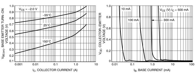
Figure 5. Base Emitter Turn-On Voltage vs. Collector Current
