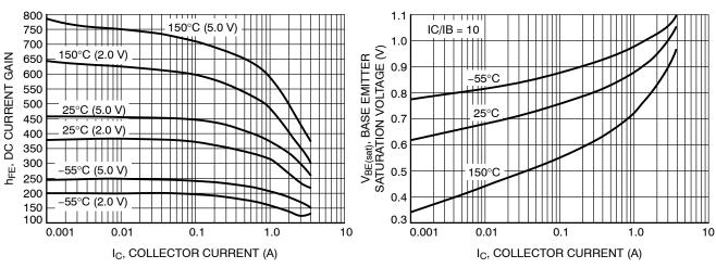
Figure 3. DC Current Gain vs. Collector Current
