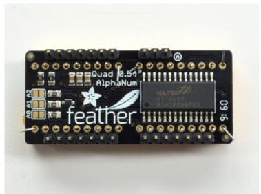
Flip over the kit and bend a few of the LED matrix legs out to keep the LED from slipping out while you solder
