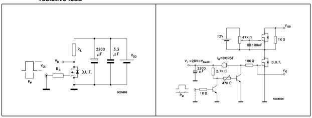
Figure 16. Test circuit for inductive load switching and diode recovery times
