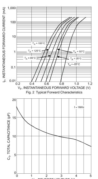
V<sub>R</sub>, REVERSE VOLTAGE (V) Fig. 4 Typical Total Capacitance
