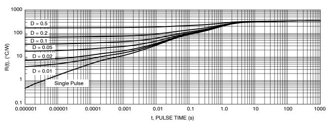
Figure 14. Transient Thermal Resistnce
