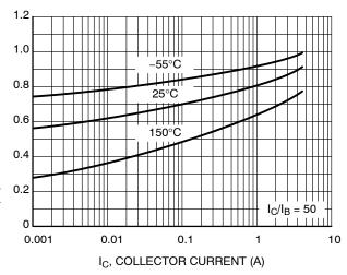
Figure 7. Base-Emitter Saturation Voltage
