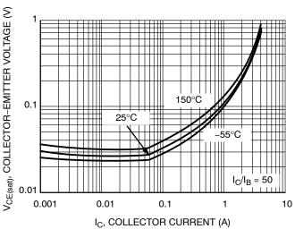
Figure 5. Collector-Emitter Saturation Voltage
