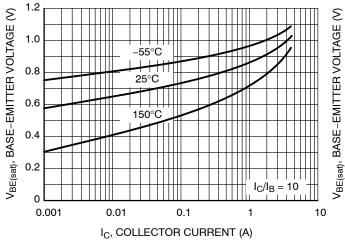
Figure 6. Base-Emitter Saturation Voltage
