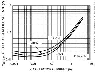
Figure 4. Collector-Emitter Saturation Voltage
