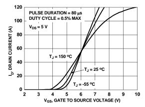
Figure 5. Transfer Characteristics
