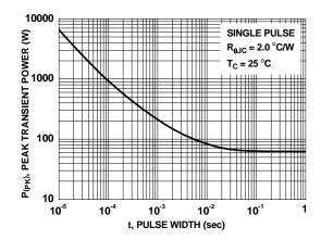
Figure 12. Single Pulse Maximum Power Dissipation
