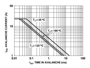
Figure 9. Unclamped Inductive Switching Capability
