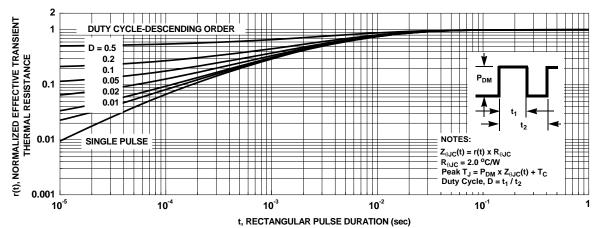
Figure 13. Junction-to-Case Transient Thermal Response Curve
