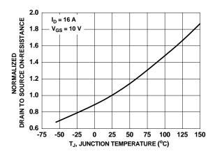
Figure 3. Normalized On-Resistance vs. Junction Temperature
