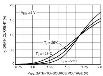
Figure 2. Transfer Characteristics
