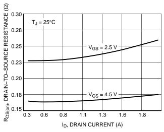
Figure 4. On–Resistance vs. Drain Current and Gate Voltage
