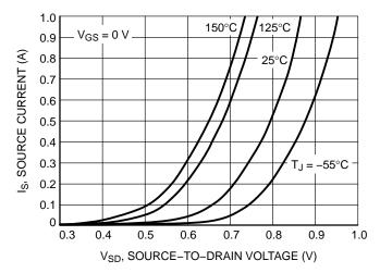
Figure 9. Diode Forward Voltage vs. Current
