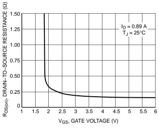
Figure 3. On-Resistance vs. Gate-to-Source Voltage
