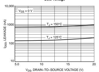
Figure 6. Drain-to-Source Leakage Current vs. Voltage
