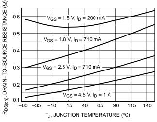
Figure 5. On–Resistance Variation with Temperature
