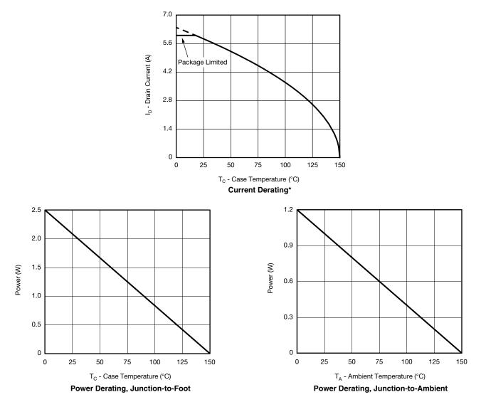
\* The power dissipation P<sub>D</sub> is based on T<sub>J(max.)</sub> = 150 °C, using junction-to-case thermal resistance, and is more useful in settling the upper dissipation limit for cases where additional heatsinking is used. It is used to determine the current rating, when this rating falls below the package limit.
