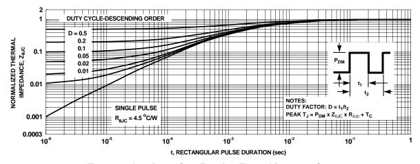
Figure 13. Junction-to-Case Transient Thermal Response Curve
