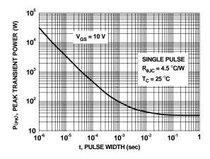
Figure 12. Single Pulse Maximum Power Dissipation
