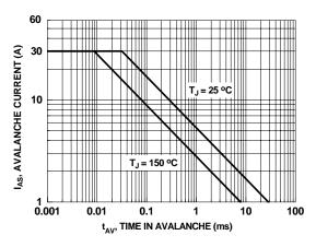
Figure 9. Unclamped Inductive Switching Capability
