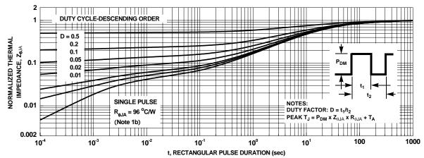
Figure 14. Junction-to-Ambient Transient Thermal Response Curve
