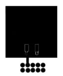
a) 40 °C/W when mounted on a 1 in<sup>2</sup> pad of 2 oz copper
