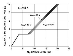
Figure 7. Gate Charge Characteristics
