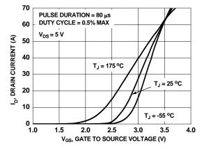
Figure 5. Transfer Characteristics
