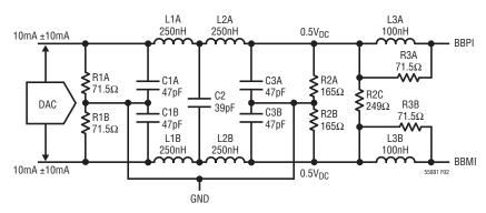
Figure 2: Baseband Interface with 5th-Order Filter and 0.5V<sub>CM</sub> DAC (Only I Channel is Shown)
