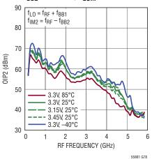
Output IP2 vs RF Frequency for Low Side LO Injection ( $f_{BB1} = 140$ MHz,  $f_{BB2} = 141$ MHz,  $P_{LOM} = 0$ dBm
