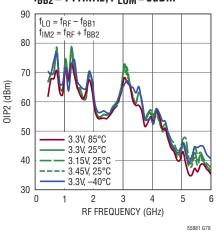
Output IP2 vs RF Frequency for Low Side LO Injection ( $f_{BB1}$  = 140MHz,  $f_{BB2}$  = 141MHz,  $P_{LOM}$  = 10dBm
