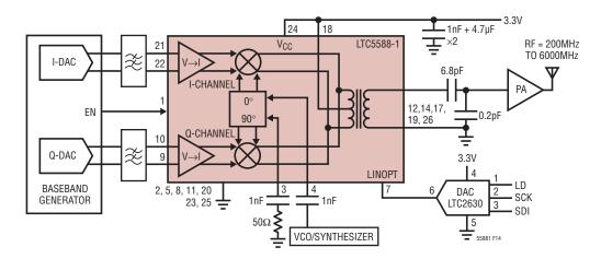
Figure 14. 200MHz to 6000MHz Direct Conversion Transmitter Application
