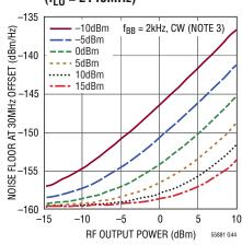
**Output Noise Floor vs RF Output Power and Differential LO Input** Power  $(f_{L0} = 2140MHz)$
