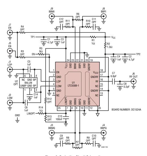
Figure 8. Evaluation Circuit Schematic
