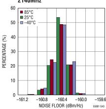
**Output Noise Floor vs RF Output** Power and LOM Port Input Power  $(f_{LO} = 2140MHz)$
