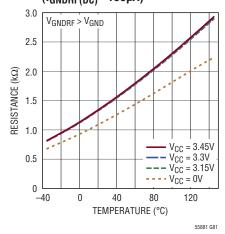
GNDRF to GND Thermistor DC Resistance vs Temperature  $(I_{GNDRF(DC)} = 200\mu A)$
