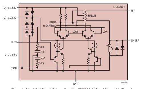
Figure 1. Simplified Circuit Schematic of the LTC5588-1 (Only I Channel is Shown)
