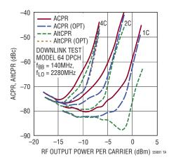
Figure 12. ACPR, AltCPR and ACPR, AltCPR with Optimized LINOPT Voltage vs RF Output Power at 2.14GHz for W-CDMA 1, 2 and 4 Carriers
