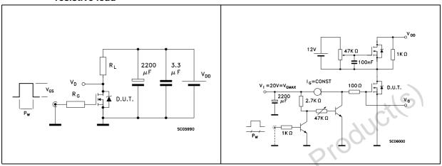
Figure 14. Test circuit for inductive load switching and diode recovery times
